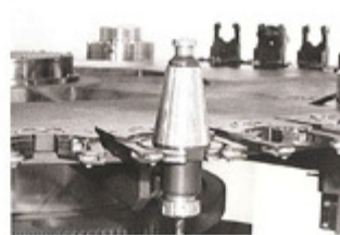
Live tool in axial setting
